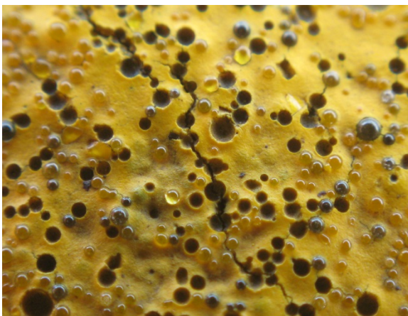
Premature Bead Loss: Incorrect or no bead coating on glass beads.
